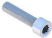
Allen screw M8X100 DIN912 A2
