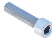
Allen screw M8X35 DIN912 A2
