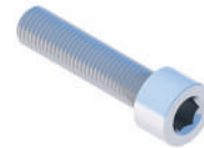
Allen screw M8X35 DIN912 A2
