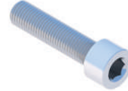
Allen screw M8X35 DIN912 A2
