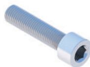
Allen screw M8X35 DIN912 A2
