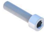
Allen screw M8X100 DIN912 A2
