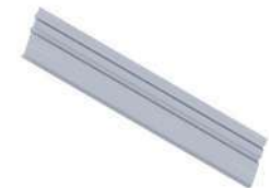
Windchest South support L=2175/2355/2703mm
