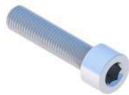
Allen screw M8X100 DIN912 A2
