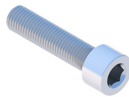
Allen screw M8x100 DIN912 A2 SIM8x100A2
