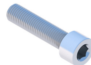
Allen screw M8X35 DIN912 A2
